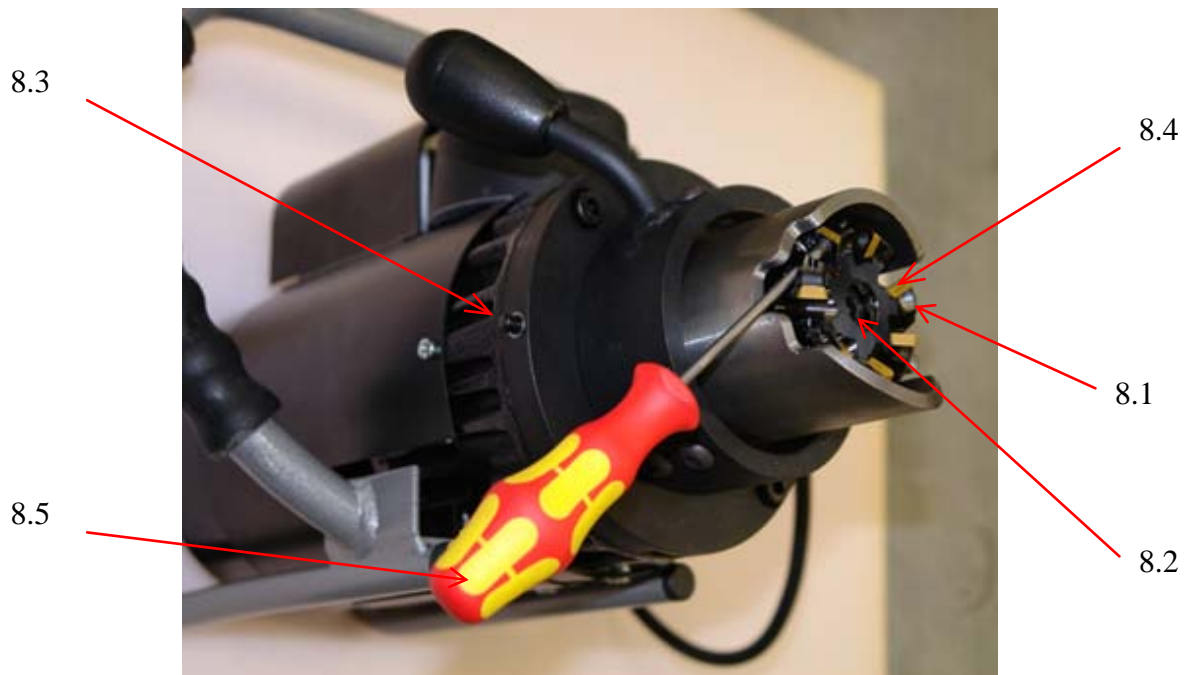
Fig.8 - Exchange of milling head and machining inserts
