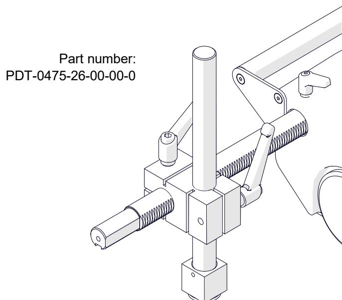
To install, loosen the handle of the torch holder and remove the holder. Then, put the support onto the rack, tighten with the handle, and install the holder again.
