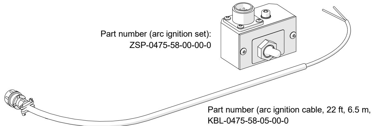
Install with the 4 mm hex wrench as shown in the figure. Plug the cable into the socket. Refer to the diagram from the figure and connect one brown wire to one terminal of the cutting circuit. Then, connect the blue wire to the other terminal of the same circuit.
