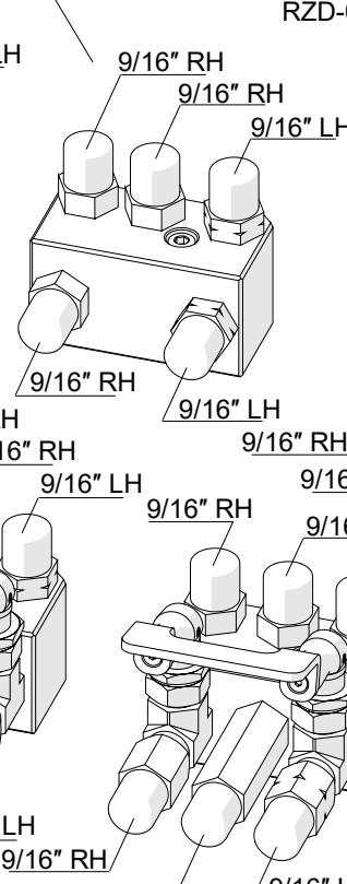
2/2 manifold with cut off valve (imperial):
