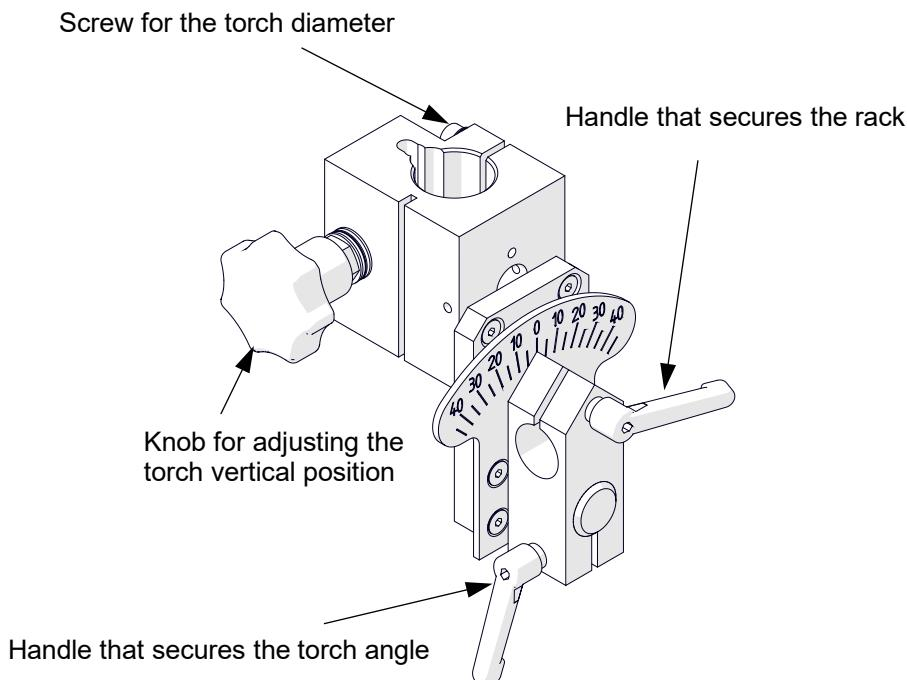
The precise machine torch holder allows torches with the diameter of 1 3/8" (35 mm) equipped with a rack. Loosen the lower handle to precisely set the torch angle. Use the knob to adjust the vertical position of the torch.
