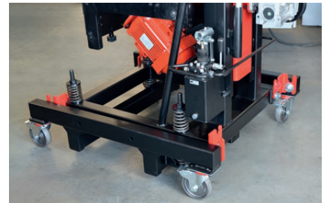
Dedicated trolley. Locks to stiffen machine for stationary work unlocks for easy movement in workspace.
