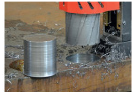
Drilling Capacity up to 5" (127 mm) Max Depth of cut up to 4" (100 mm)
