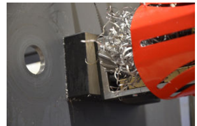
Swivel base for more precise drilling
