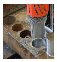
Milling capacity up to 4"(100 mm) Max depth up to 4" (100 mm) Max stroke up to 9" (225 mm)
