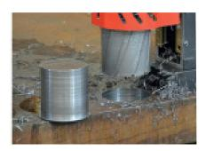
Drilling Capacity up to 6" (152 mm) Max Depth of cut up to 4" (100 mm)
