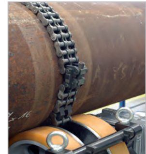
Adjustable chain (ø 8" - 40") ensures positive axial rotation
