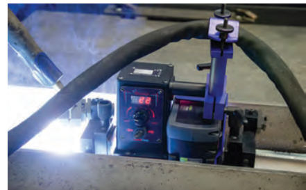
Easily place torch on either side of carriage
