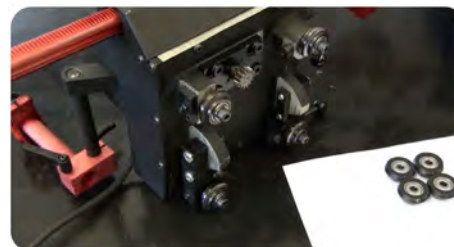
Set of Hi Flex Rail Guiding Rollers (4 pcs) Product code: SM-ZSP-0673-07-00-00-0
