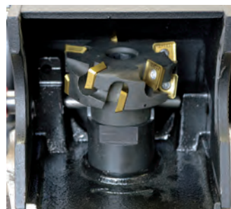
Mono block milling head, with 10 indexable inserts.
