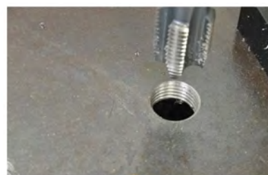
Through and Blind hole tapping
