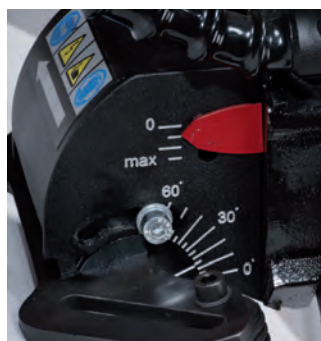
Continuous angle adjustment from 0 to 60 degrees.
