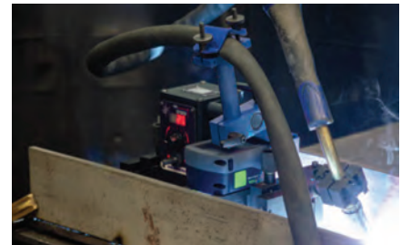
Easily place torch on either side of carriage
