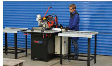
Auxiliary tables to accommodate long workpieces
