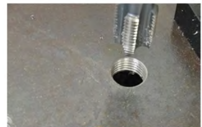
Through and Blind hole tapping
