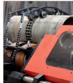
Clamping device for short pipes of 15-3/4" - 32-11/16" length
