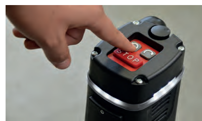
Counterclockwise (CCW) rotation User-friendly control of tapping tool release
