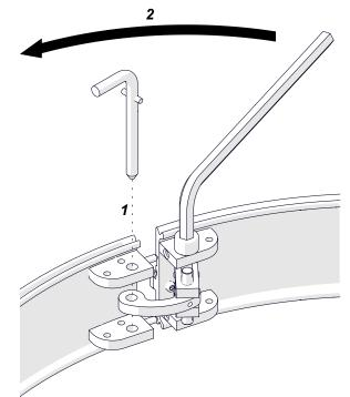
Use the 13 mm flat wrench to adjust the bolts (or the screws by hand) until they are in contact with the workpiece (1). Adjust each support equally to make the track concentric to the workpiece. Lock the supports with the nuts (2) or levers.
