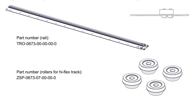
Use the 13 mm flat wrench to remove the standard rollers and install the rollers for hiflex track.
