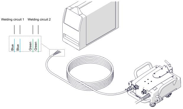
Make sure that the arc ignition cable is connected correctly. To do this, turn on the power of the carriage, and then set the arc ignition switch to TEST. This should enable the arc for a while.
