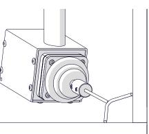
The figure shows how the tracking system works. When the tip of the sensor moves, the system senses any small change in position of the seam. Then, the oscillator, the vertical slide, and the torch, are moved to maintain the correct position above the seam.
