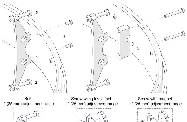
Put the workpiece vertically, and then put the rails onto the workpiece so that the teeth of the racks point down. Next, for all rails, use the 12 mm hex wrench to set the hinge as shown. Then, put the lock pin through the holes (1), and then rotate the wrench (2) to connect the rails.
