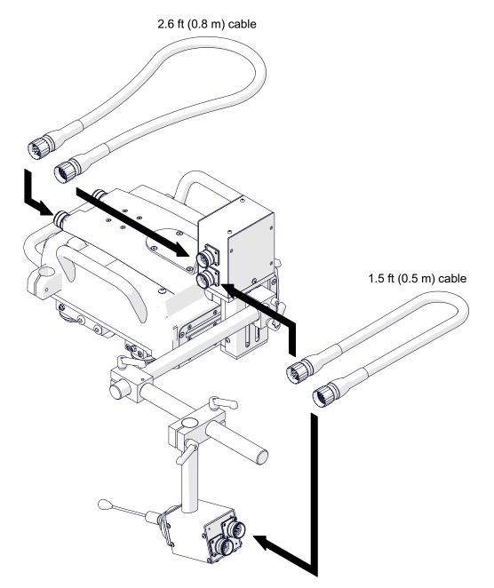
Install the torch into the torch holder. Then, tilt the rod of the sensor against the workpiece so that there is tension in the rod. Next, put the tip as shown.
