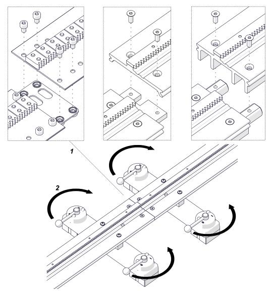
If a semi-flex rail is put on a curve, before you attach more rails use the 4 mm hex wrench to loosen the screws of the connecting plates (1) and of the racks (2). Next, attach the rails, clamp them with levers, and then tighten the connecting plates. Put the rack adjustment tool (not included) into the hole (3), and rotate the tool to the left (4) to remove the gap (5) between the racks. Then, tighten the leftmost screw and the rightmost screw of each rack (2).
