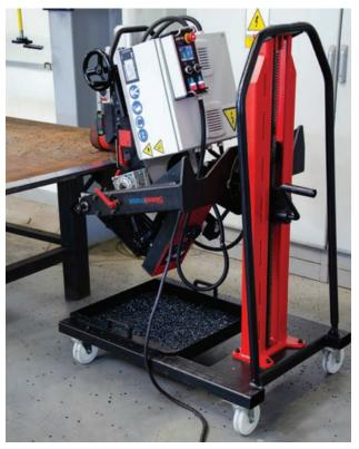
The remote pendant allows the operator to optimally adjust spindle and travel speeds for beveling ferrous and non-ferrous materials – up to 450,00 psi tensile strength.
