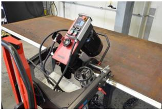
The **ABM50** creates bevels with a maximum bevel width of 2" (50 mm) at 45 degrees.
