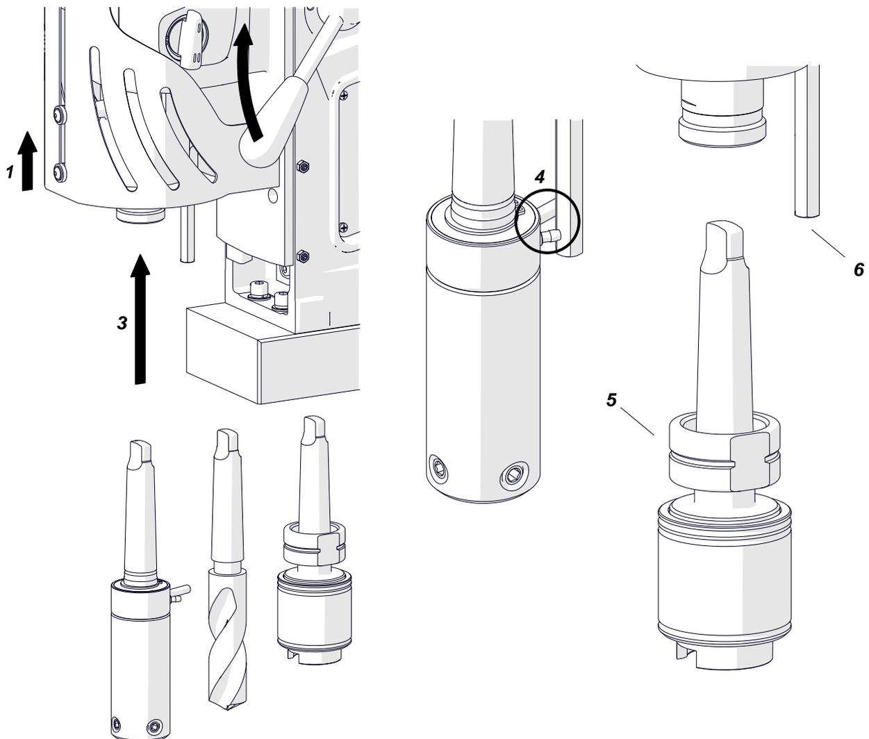
To remove the arbor (drill bit, tap chuck), continue as follows. If the arbor (tap chuck) has a nut (1), remove the nut. Next, lift the motor and rotate the spindle (2) to align the holes in the spindle and gearbox (3). Put the drift into the hole (4). Next, hold the carrying handle with one hand and hit the drift with a mallet (5).
