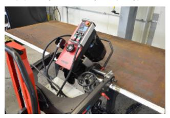
The **ABM50** creates bevels with a maximum bevel width of 2" (50 mm) at 45 degrees.
