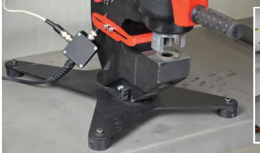
Free Standing Base for Punch SM-ZST-0507-91-00-00-0 With Foot Petal Activation for bench top operation
