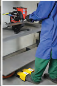
Free Standing Base for Punch SM-ZST-0507-91-00-00-0 With Foot Petal Activation for bench top operation
