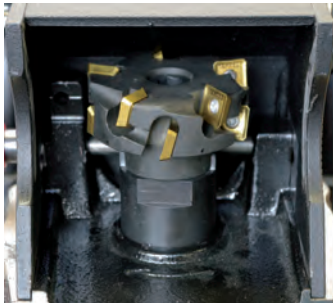
Mono block milling head, with 10 indexable inserts.
