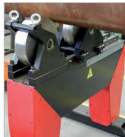
Optional heavy-duty pipe support with 11-ton capacity
