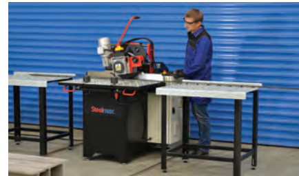
Auxiliary tables to accommodate long workpieces
