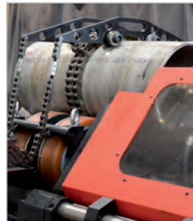
Clamping device for short pipes of 15-3/4" – 32-11/16" length
