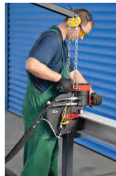
Overhead Support for Punch SM-ZUR-0517-15-00-00-0
