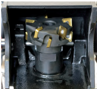
Mono block milling head, with 10 indexable inserts.
