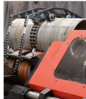
Clamping device for short pipes of 15-3/4" – 32-11/16" length
