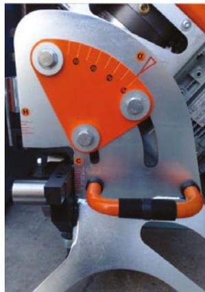
Infinitely adjustable angle between 15 and 50 degrees
