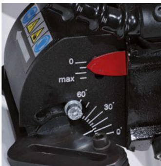
Continuous angle adjustment from 0 to 60 degrees.
