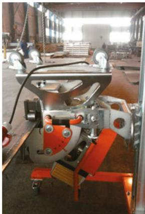
Rotates 180 degrees for bottom side bevel.
