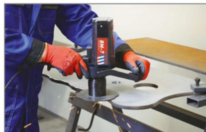
Contour edge beveling and radius milling
