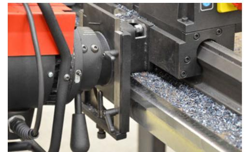
Beveling greater lengths of plate is accomplished with additional sections of guide tracks.
