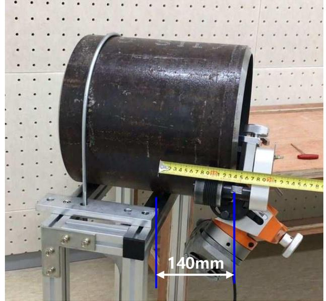
1. Loosen the Inner Roller Adjustment Handle and Outer Roller Adjustment Handle sufficiently so that the pipe will slide easily between the Inner Roller and Outer Roller.
