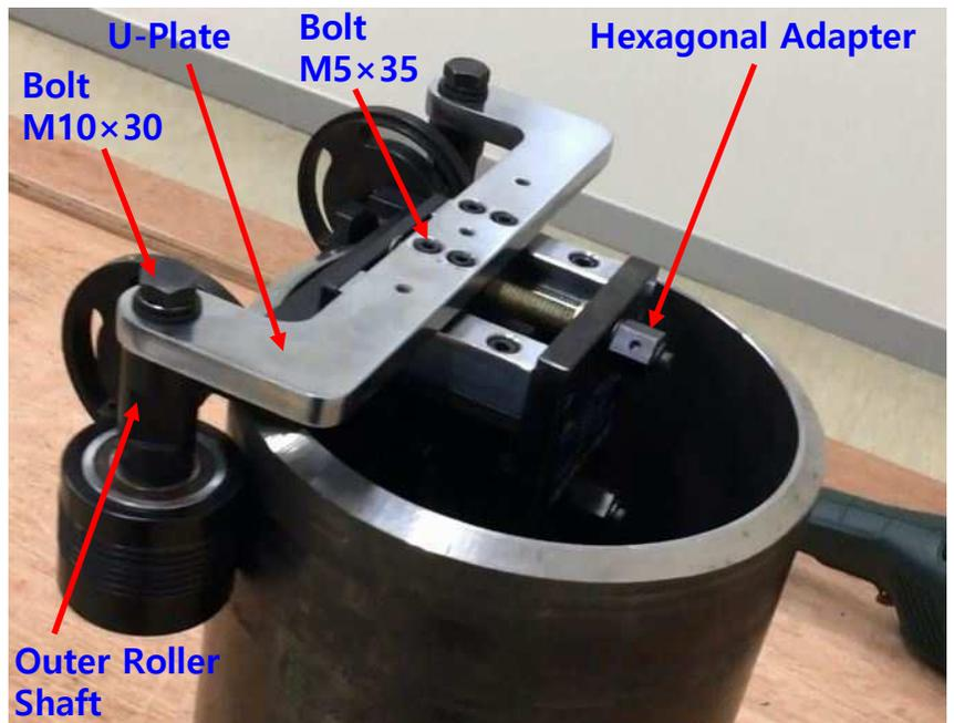
5. Assemble the U-Plate and Outer Roller Shaft Assembly to the Support Block by securing the four M5 x 35 bolts.
