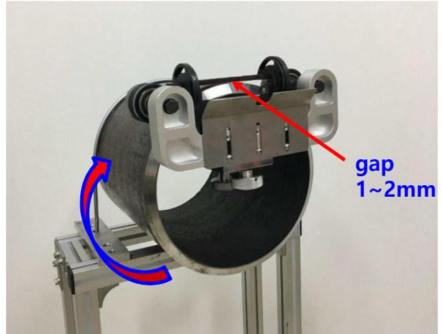
4. With the machine at the top of the pipe, the Chamfer Mill can be installed.
