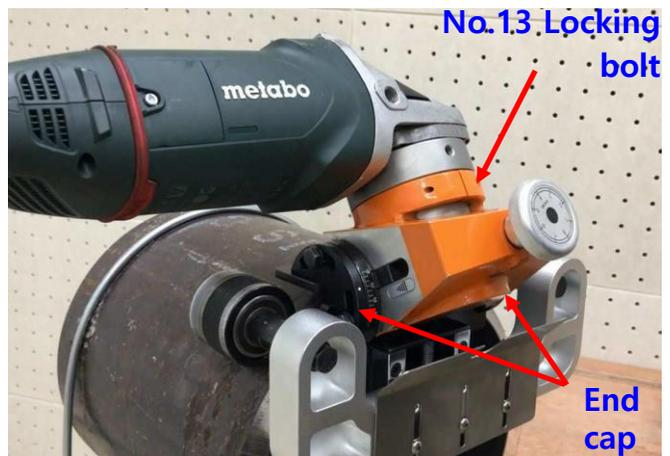
6. Insert the two Operator Handles on both sides to the Outer Roller Shaft. If it is difficult to insert the Handle because the position of the motor is not appropriate, loosen the Locking Bolt, adjust the position of the Handle and then tighten the Locking Bolt again.
