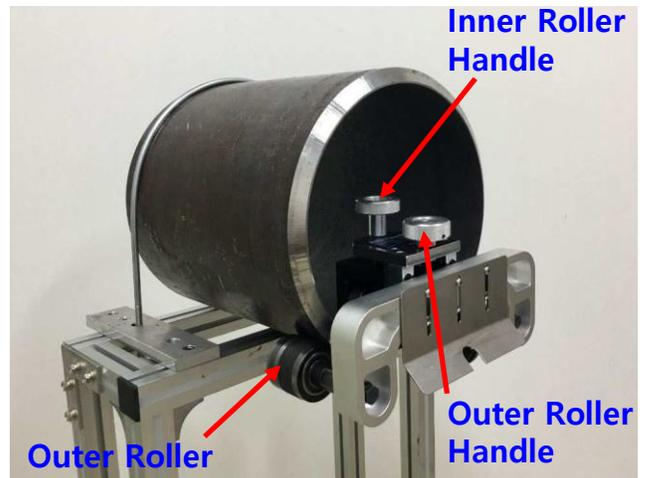
3. Rotate the unit clockwise to the top of the pipe to check alignment and fit of the unit to the pipe. After tightening the Outer Roller Adjustment Handle, there should be a gap between the surface of the outside diameter of the pipe and lower portion of X-Plate of 1-2mm. If the gap is smaller than this, adjust the gap by further tightening the Outer Roller Adjustment Handle to achieve the desired gap.
