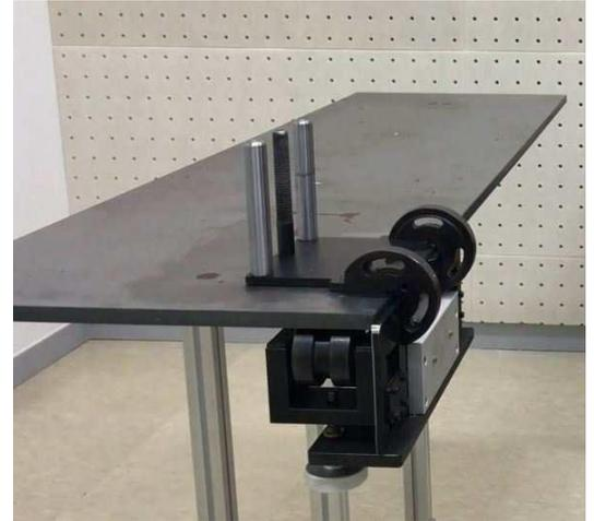
\*Before inserting the fixing bracket onto the plate, confirm that the Inner Roller Adjustment Handle is sufficiently loose to provide enough gap so that two (2) units of Inner Rollers can be inserted onto the plate.
