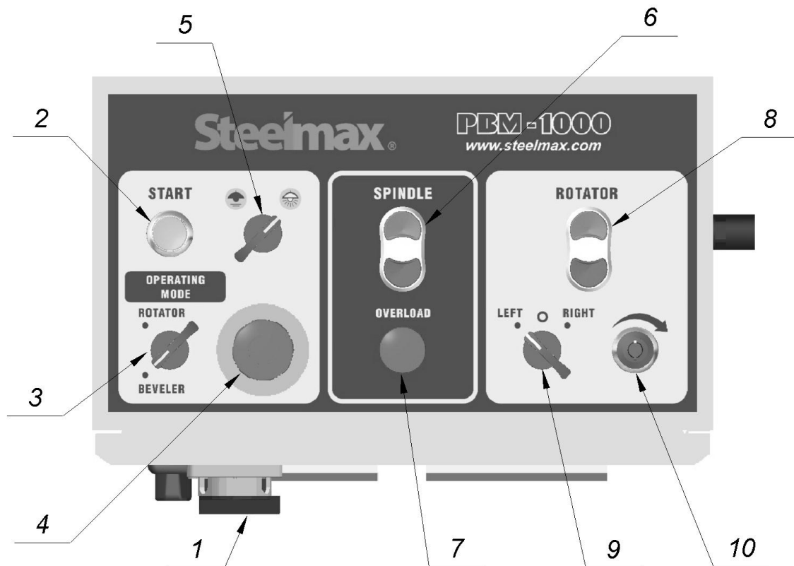
Figure 4. Control panel design: 1 – main switch, 2 – control button, 3 – operating mode lever, 4 – emergency button, 5 – work area light, 6 – spindle start/stop button, 7 – lamp indicating spindle overload, 8 – rotator start/stop button, 9 – rotation direction switch, 10 – rotator speed adjusting knob
