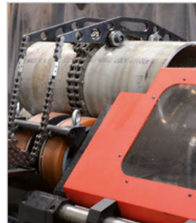
Clamping device for short pipes of 15-3/4" - 32-11/16" length
