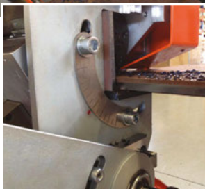
Rapid 180° inversion for bottom side bevel
