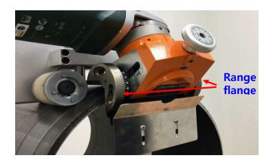
(If the bevel depth value is not set at or below zero (0) level at installation, it may cause damage to the machine and possible injury to the operator.)
