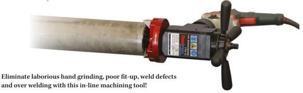
Extremely productive when full penetration welding is required, the Steelmax **PB5** will produce accurate weld preparation within seconds. Creating highly repeatable and consistent fit-up, this tool dramatically reduces cycle times and improves work flow. By utilizing a self-centering mandrel which mounts internally to the open end of the tube or pipe, the PB5 can be rapidly deployed from one pipe to another.
