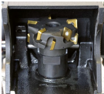
Mono block milling head, with 10 indexable inserts.
