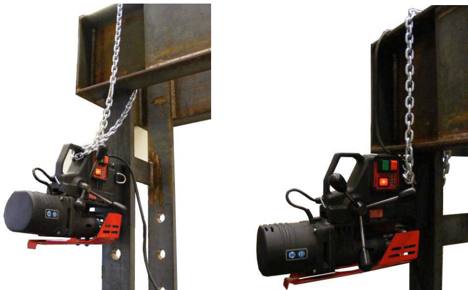
Drawing No 1 The safety chain application
