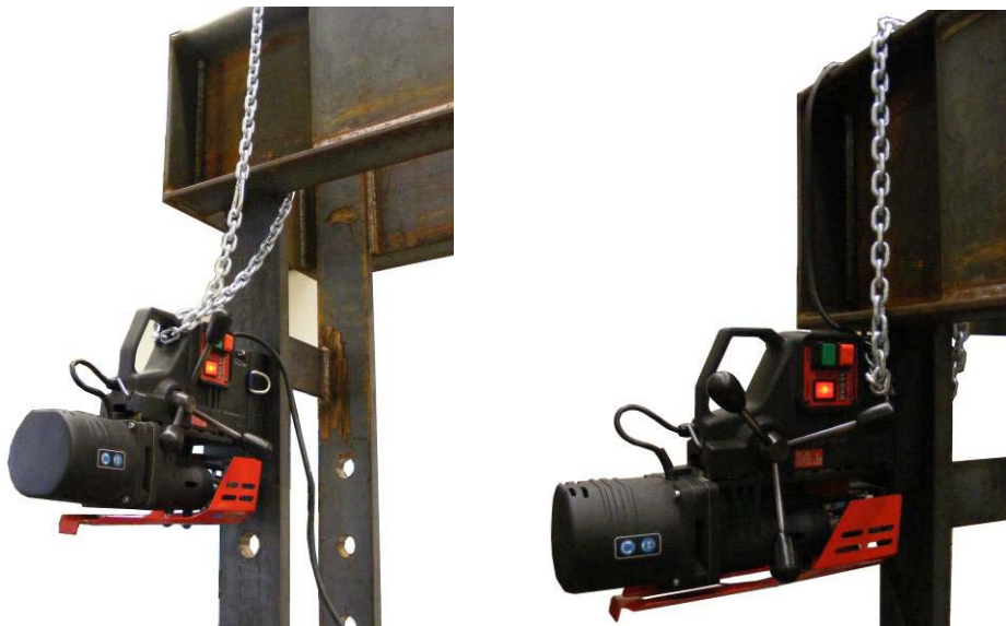
Drawing No 1 The safety chain application
